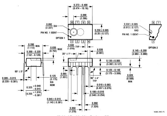
Molded Dual-In-Line Package (N) NS Package N08E
