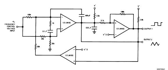
$V^* = +30 \ V_{DC}$   $+250 \ mV_{DC} \le V_C \le +50 \ V_{DC}$   $700Hz \le f_0 \le 100kHz$
